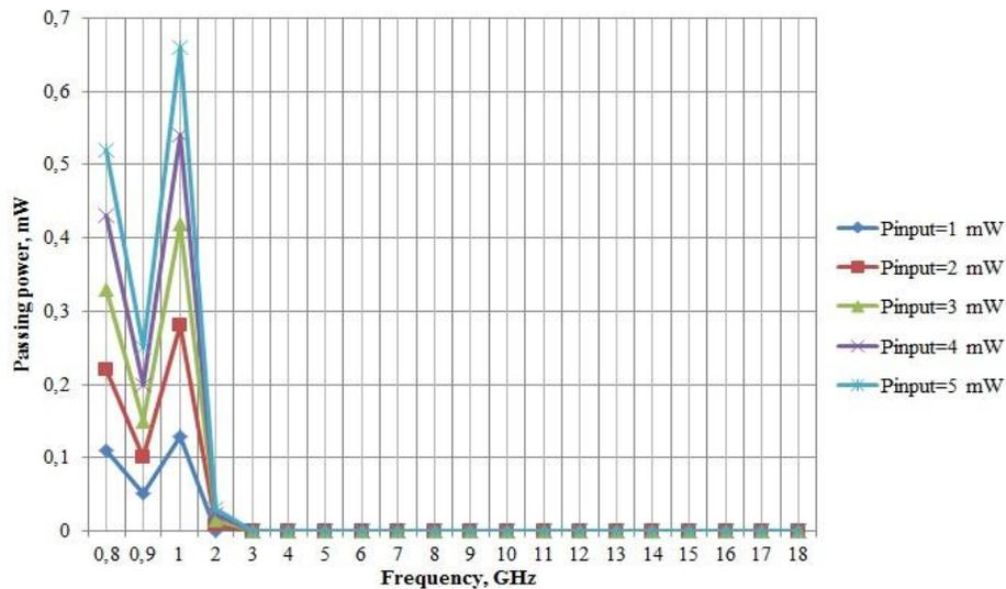
**Figure (8) Frequency dependence of the passing power in the frequency range of 0.8 ... 18 GHz for the filled pyramidal shielding module**
