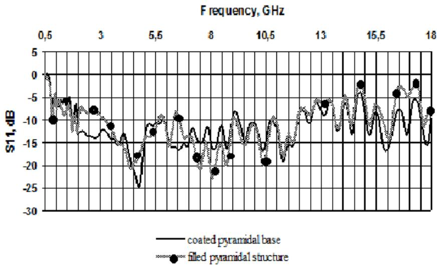
Figure (5) Frequency dependence of the reflection coefficient in the frequency range of 0.5 ... 18 GHz for the filled pyramidal shielding module
