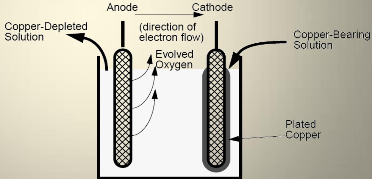
Figure4:Electrowinning process [4]
