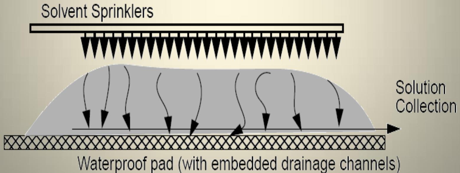
Figure3: Heap Leaching
