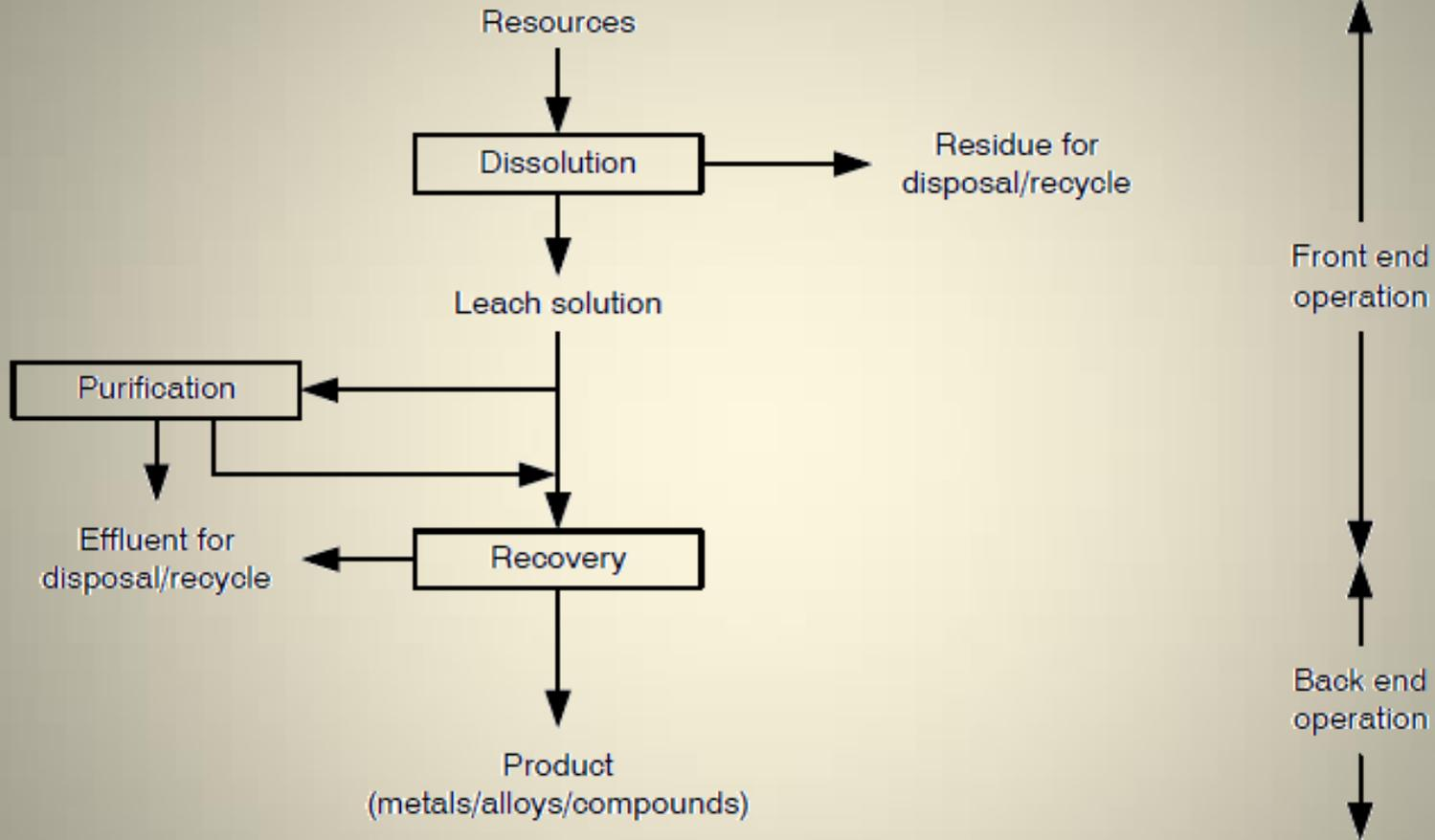
Figure 1: Basic unit processes in hydrometallurgy. [4]
