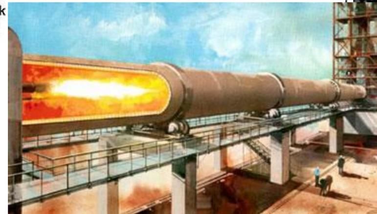
Other commercial uses of rotary kiln is cement and the removal of water from alumina
