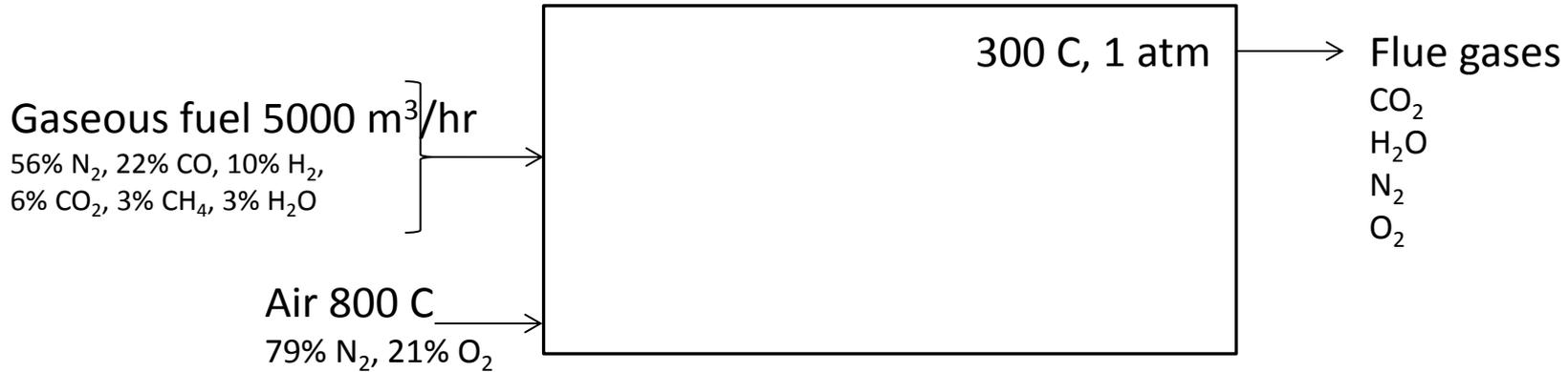
Calculate the volume of air required to burn 1 m<sup>3</sup> of regenerator gas
