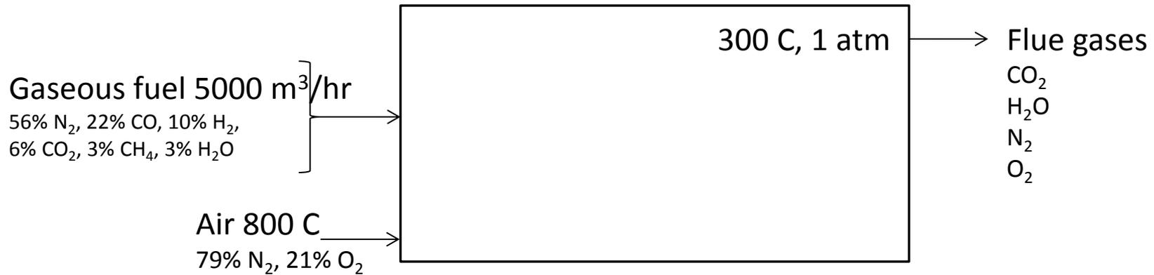
Calculate the composition of flue gases
