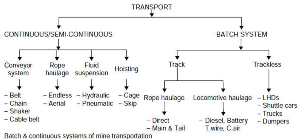
Figure 7.2 Batch and continuous system of transportation.
