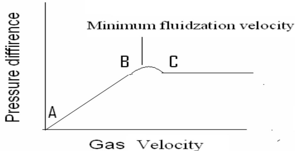
Fig. Typical Fluidization curve
