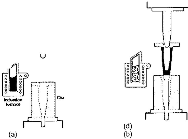
Figure : Schematic illustrating squeeze casting process
