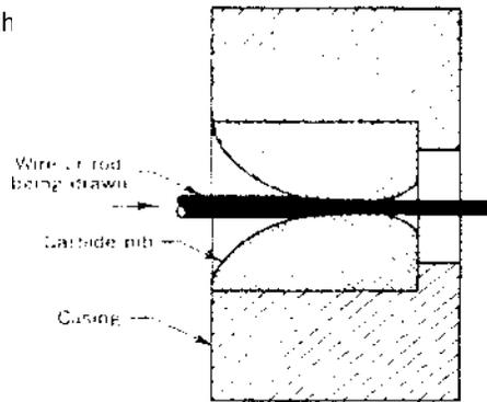
Figure 18: Section through a die used for drawing wires.
