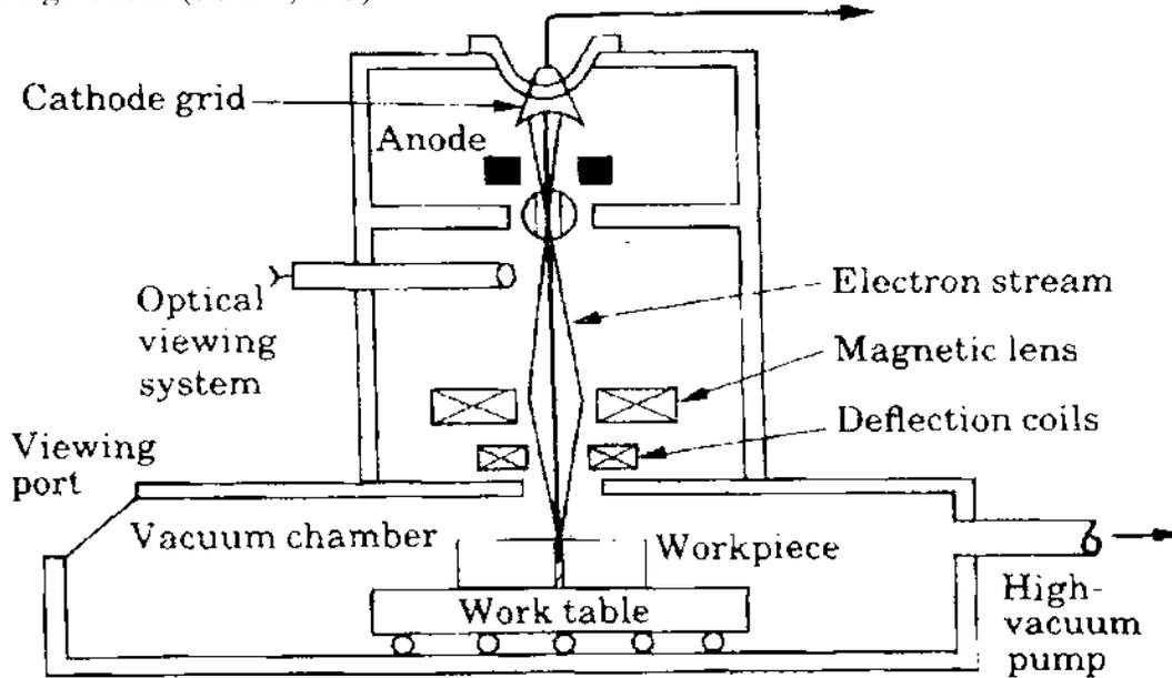
Figure : An electron beam welding process
