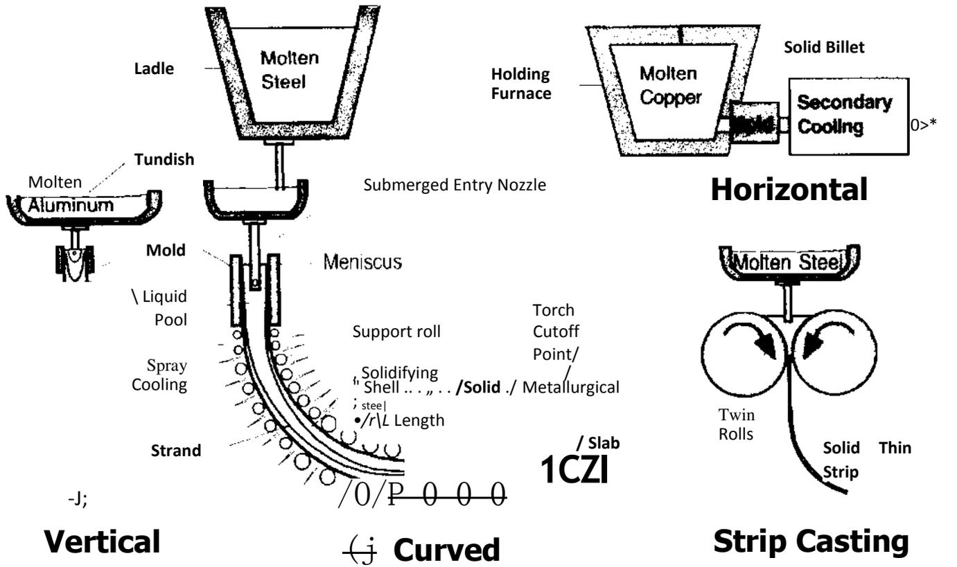
Figure 1. Various continuous casting processes
