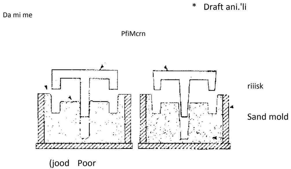
Figure 1.6 - Taper consideration in sand casting
