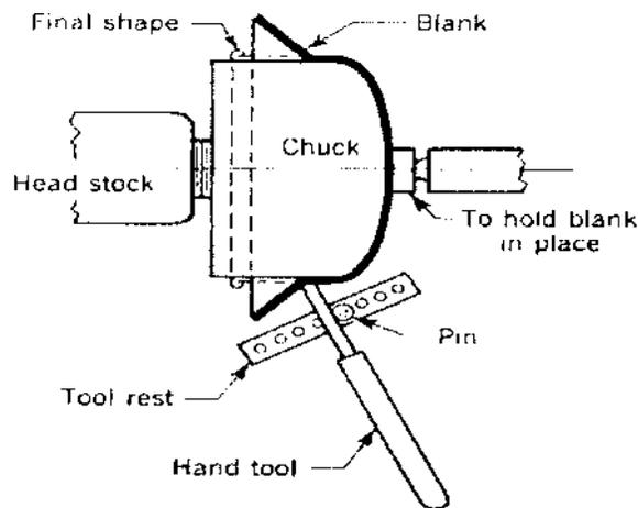
Figure 9: Metal spinning operation
