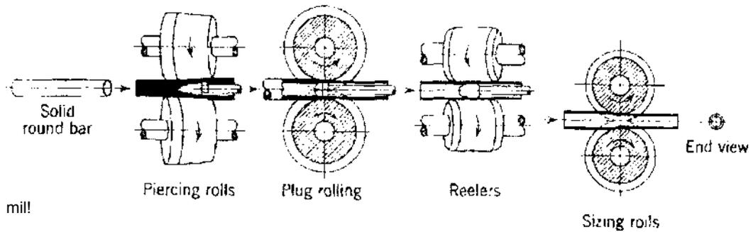
Figure 7: Principal steps in the manufacture of seamless tubing.
