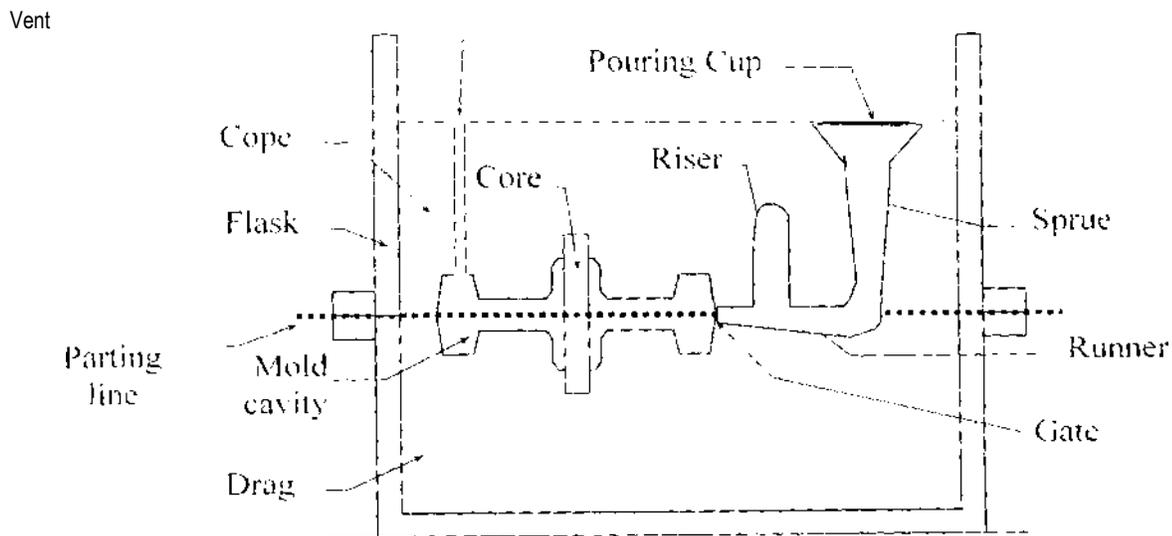
Figure 1.4 - Typical mold for a sand casting
