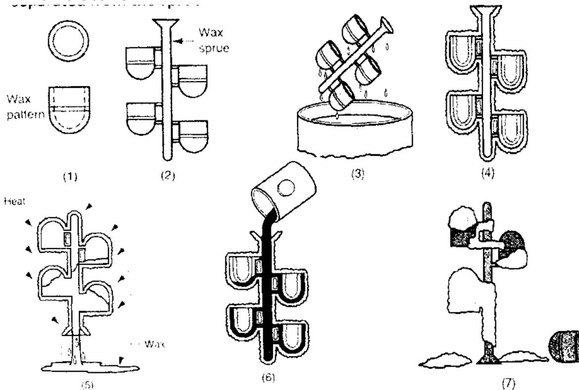
Figure.19 Steps of investment casting casting process
