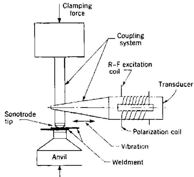
Figure ultrasonic welding
