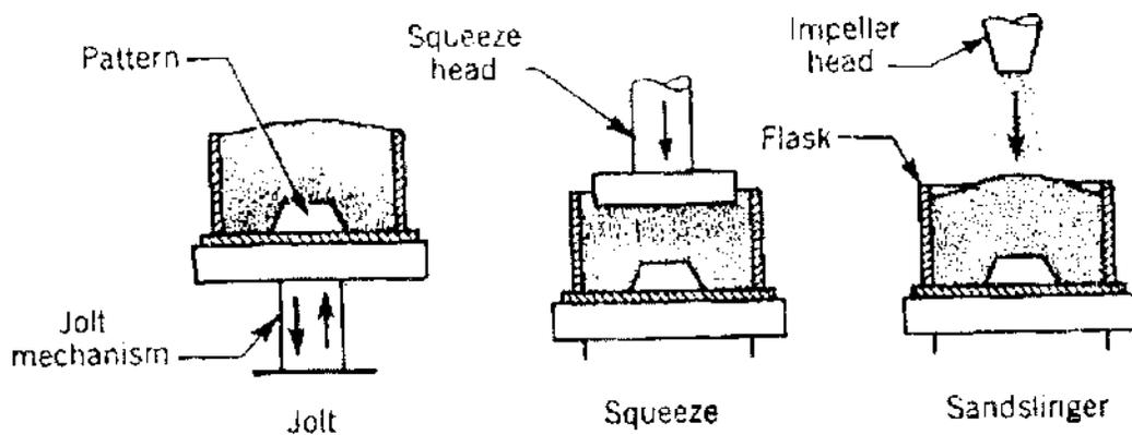
Figure 1.8- Machine molding principles
