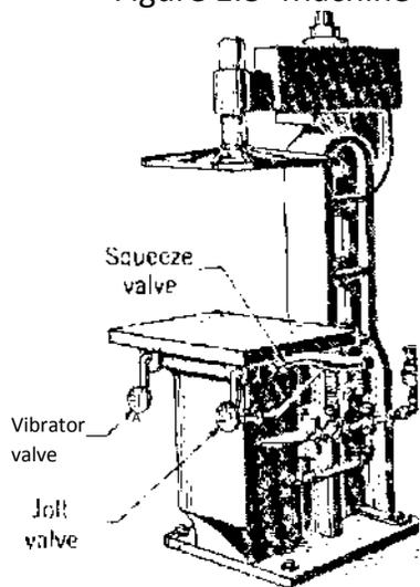
Figure 1.9 Jolt-squeeze molding machine
