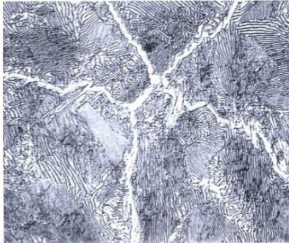
Hypo-eutectoid steel showing primary cementite along grain boundaries pearlite
