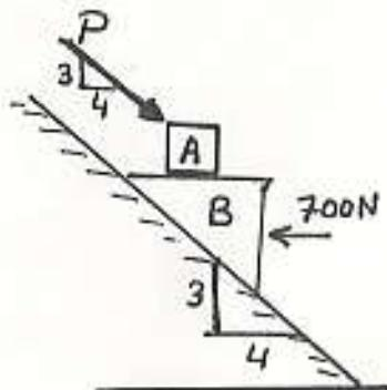
4. Three blocks are arranged as shown in figure below. The upper one is forbidden from movement by a rope. Determine the maximum value of P to impend motion. (Ans:  $P = 93.8\text{N}$ )
