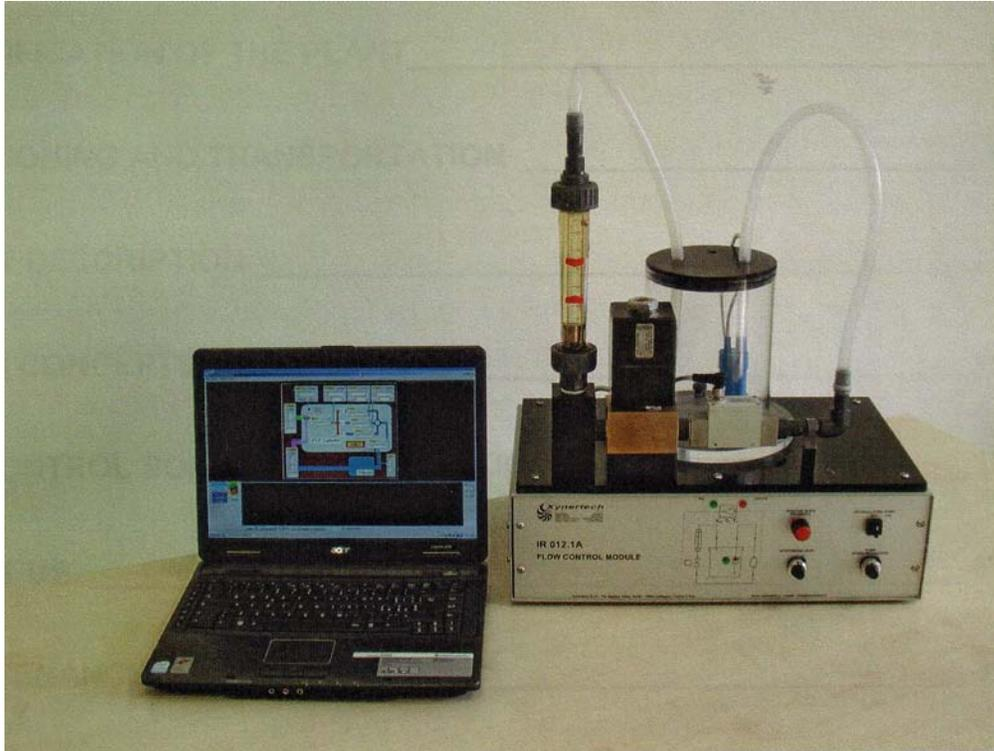
**Figure (1) On-line control of a flow system**
