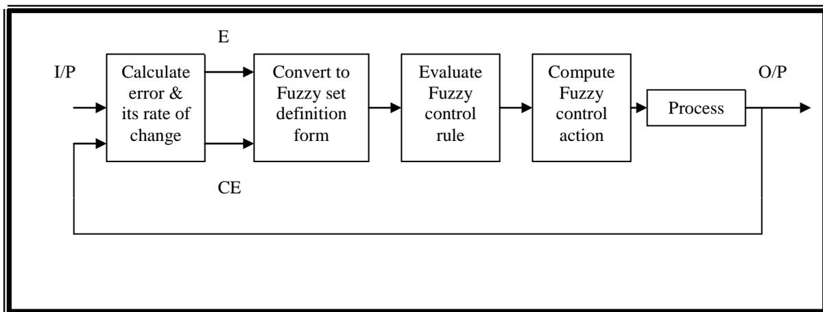
**Figure (2): Block diagram of a control system using Fuzzy Logic Control**
