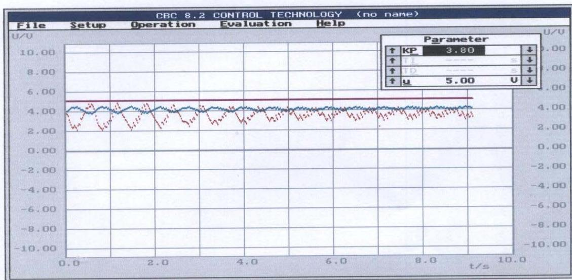
**Figure (3): Proportional Control (P) of a Flow System**
