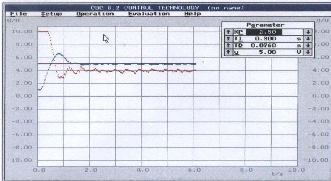
**Figure(5): Proportional-Integral-Derivative Control(PID) of a Flow System**
