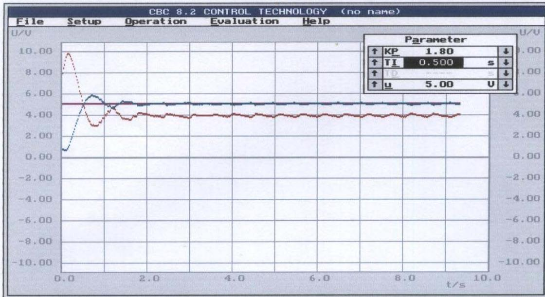
**Figure (4): Proportional-Integral Control (PI) of a Flow System**
