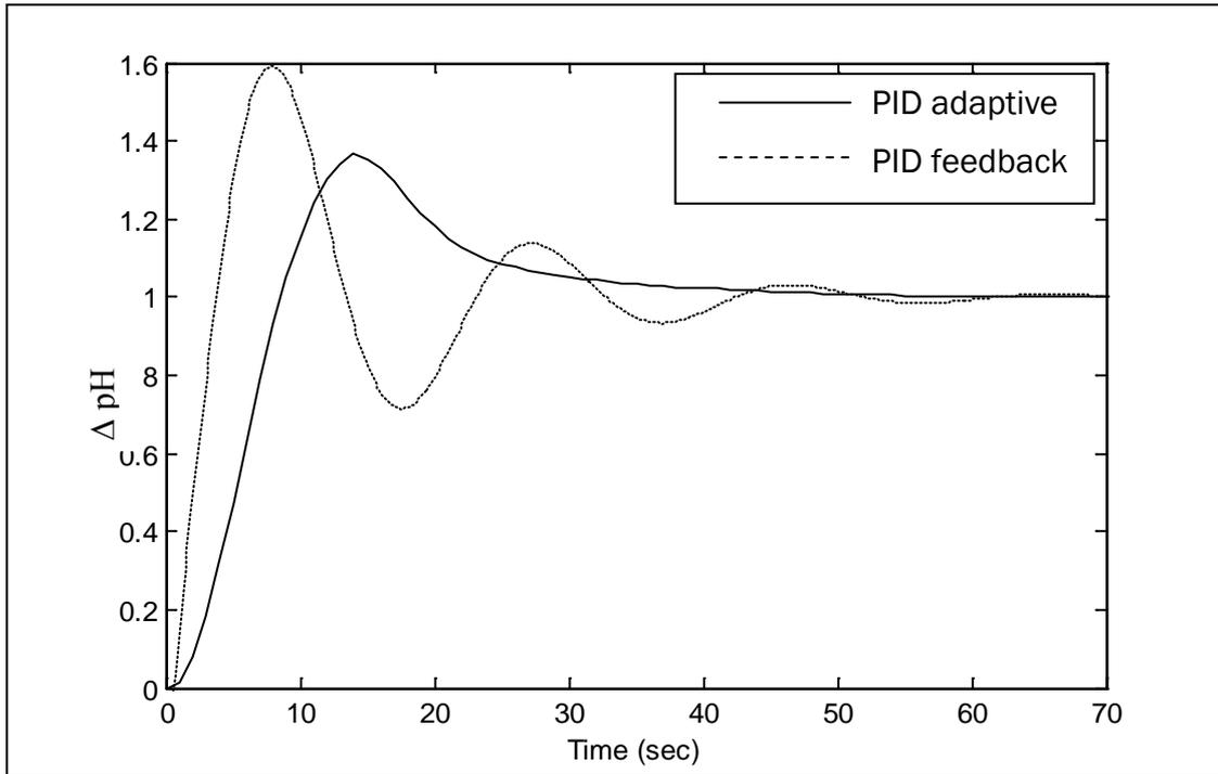
**Fig. (5) The comparison between the transient response for PID feedback controller and PID adaptive controller**
