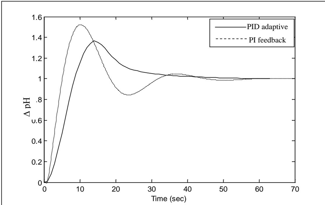
**Fig. (7) The comparison between the transient response for PI feedback controller and PID adaptive controller**
