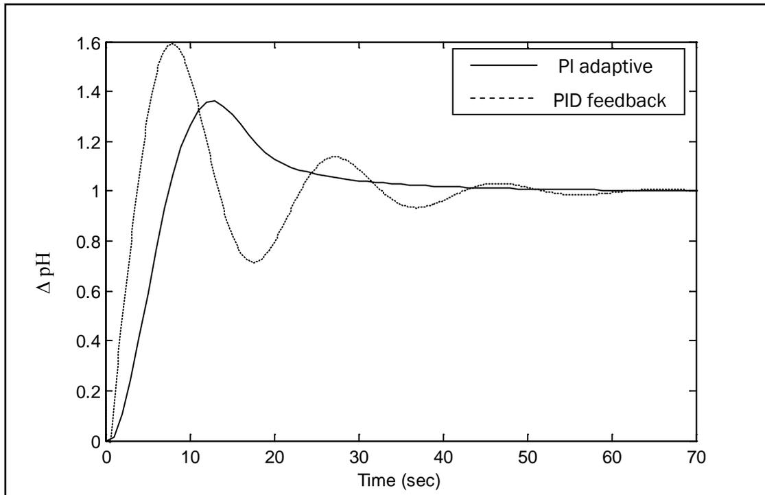
**Fig. (6) The comparison between the transient response for PID feedback controller and PI adaptive controller**
