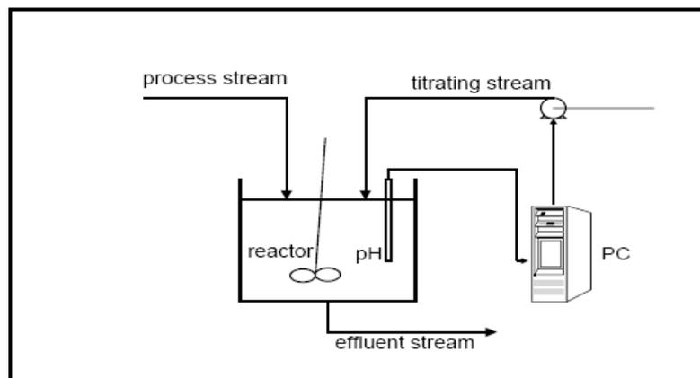
**Fig. (2) pH Neutralization Process.**
