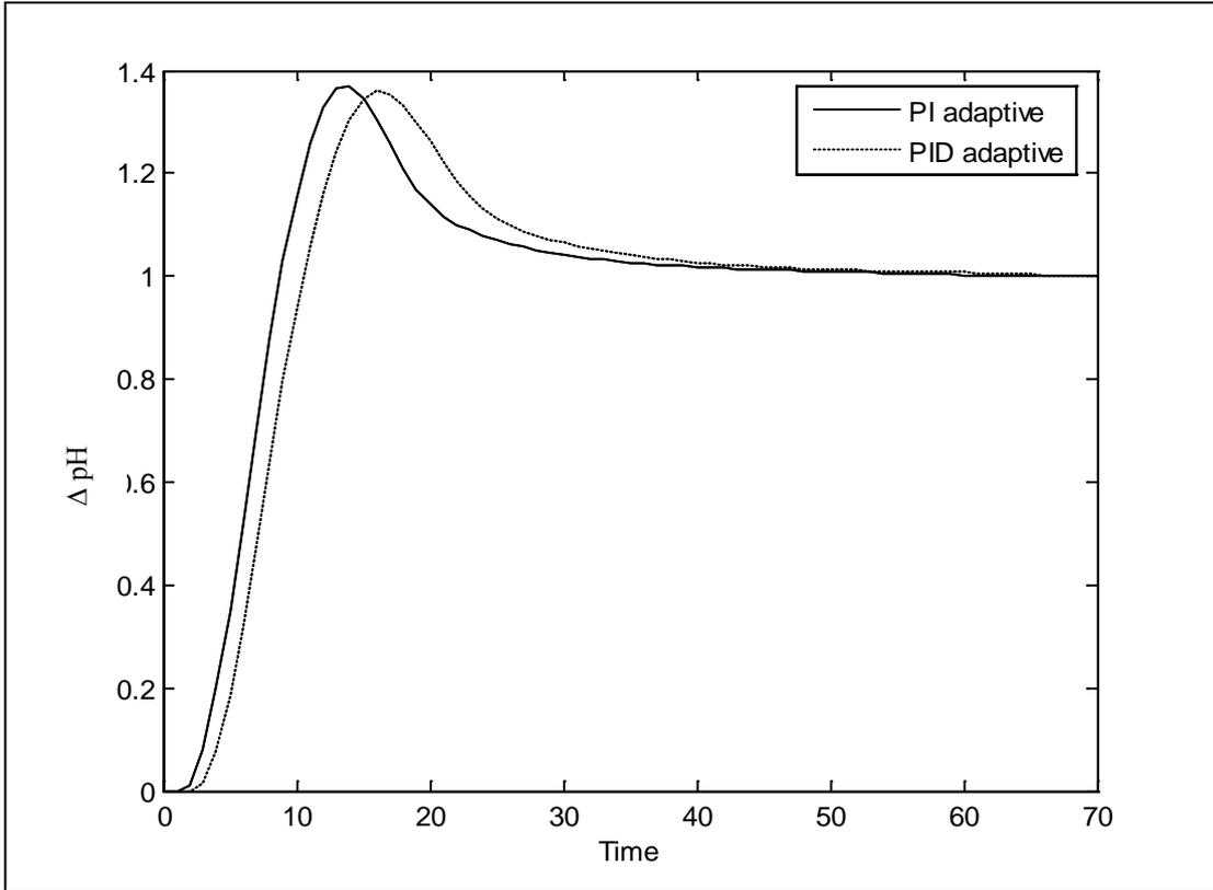
**Fig. (3) The comparison between the transient response for PI adaptive and PID adaptive controllers**
