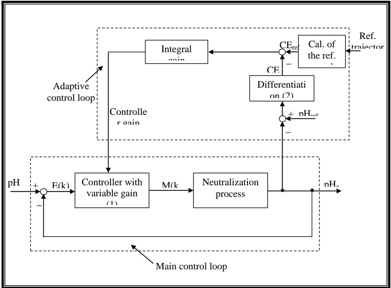
**Fig. (1) Schematic representation of the adaptive control system <sup>(9)</sup>.**
