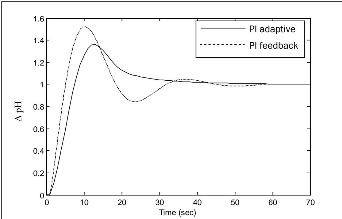
**Fig. (8) The comparison between the transient response for PI feedback controller and PI adaptive controller.**
