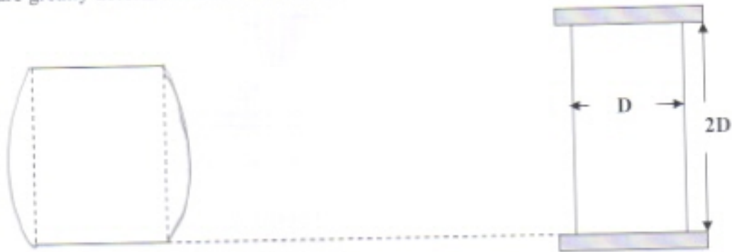
Ductile metal under the test
