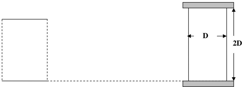
Ductile metal under the test
