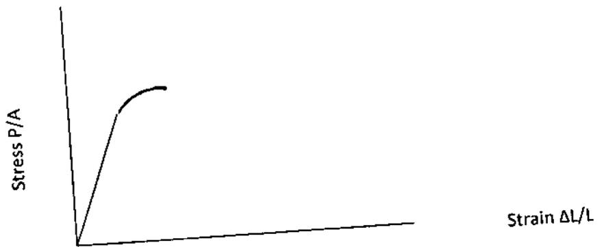
Stress - Strain curve for hard steel
