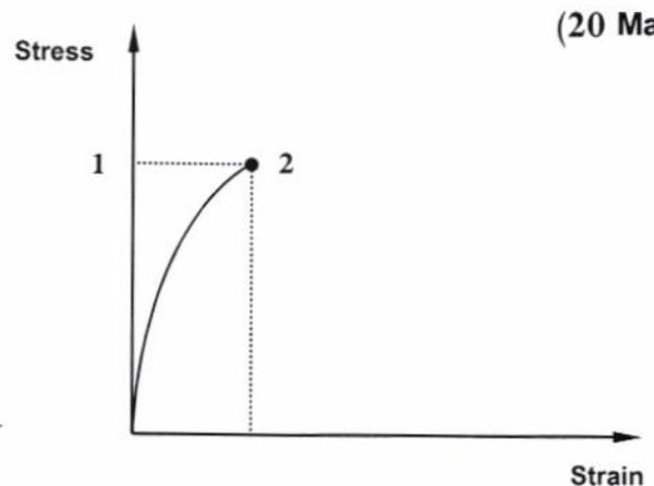
Figure 2: A stress-strain curve for a brittle material.
