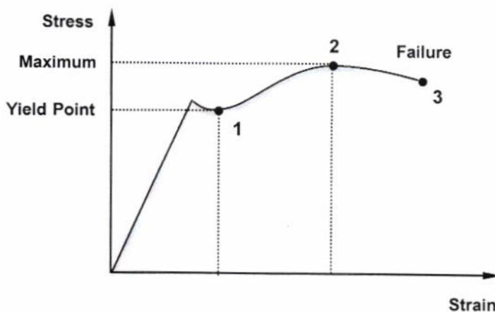
Figure 1: A stress-strain curve for a ductile material.
