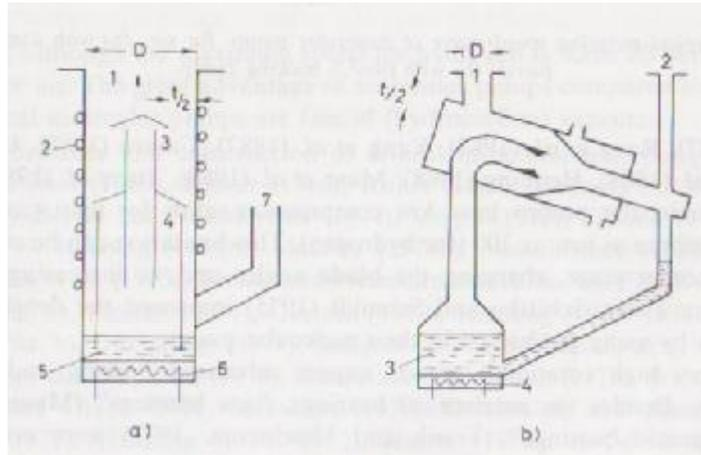
(a) diffusion pump: 1.High vacuum; 2.Water cooling; 3.First stage; 4.Second stage; 5.Pump oil; 6.Heater; 7.Fore-vacuum; (b) vapour pump; 1.Intake port; 2.Fore-vacuum; 3.Oil; 4.Heater.
