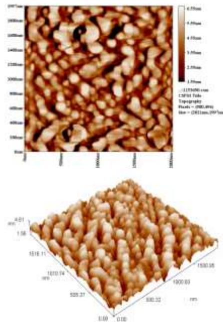
Fig. (4) AFM image of the prepared  $\text{In}_2\text{O}_3$  nanoparticles
