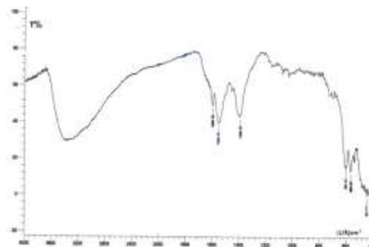
Fig. (1) FTIR spectrum of In<sub>2</sub>O<sub>3</sub> nanoparticles
