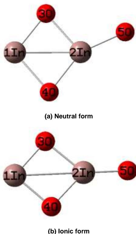
Fig. (4) Optimized structure of one unit from indium oxide
