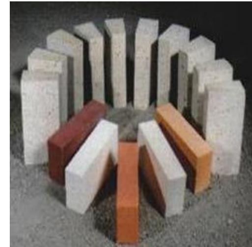
**Refractories** are materials that can withstand high temperatures without softening or deformation in shape. Refractories are mainly used for the construction of lining in - furnaces, kilns, converters, etc. The main function of a refractory is to withstand and maintain high temperatures and to resist the abrasive and corrosive action of molten metals, slags and gases.
