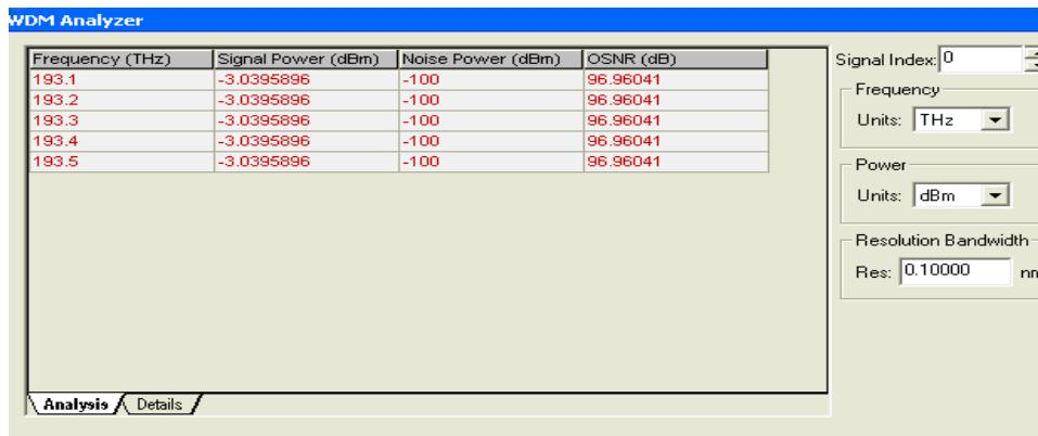
Fig.11 Properties of the WDM analyzer of the five channels
