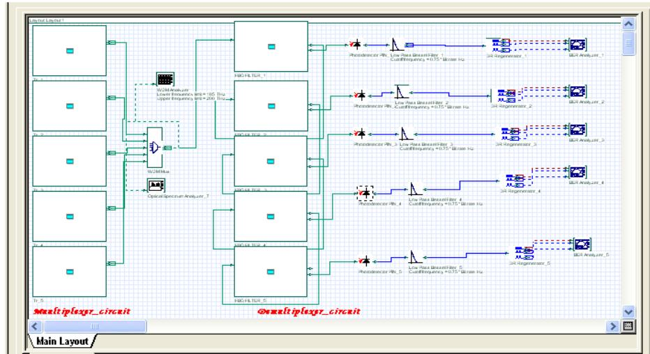
**Fig. 2 Using FBG in the WDM multiplexer /demultiplexer**
