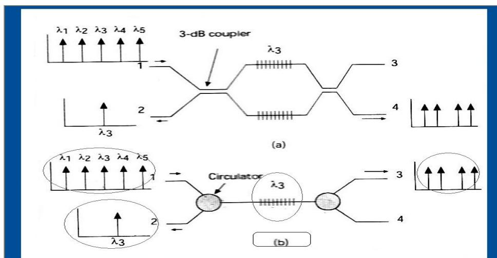
**Fig. 1 Illustration of Multiwavelength Receiver**
