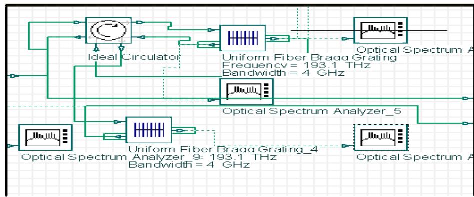
**Fig. 5 One of the demultiplexer subsystems before solving dispersion problem**
