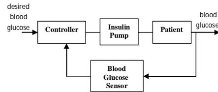
Figure 1: Closed loop insulin regulation system block diagram [2].
