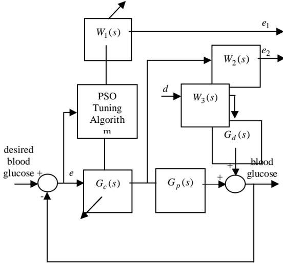
Figure 2: Block diagram of PSO based robust controller design.
