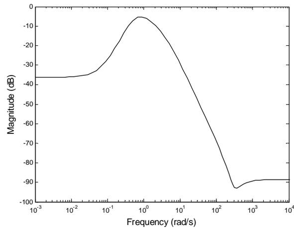
Figure 6: Frequency characteristics of the resulting robust controller.
