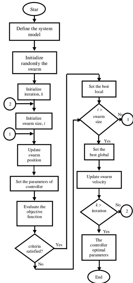
Figure 3: Flowchart of PSO based robust controller design.
